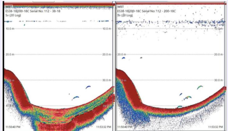
Figure 1. Echograms retrieved from Miskwabi Lake while conducting a parallel netting survey. The left image is what is 'seen' with a 38 kHz transducer, and on the right is the parallel image on a 200 kHz transducer. The larger targets seen as arcs near the bottom of the lake below 30 meters are likely lake trout. Those seen by both the 38 kHz and 200 kHz are the largest fish.
